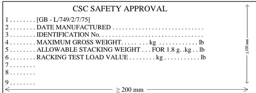
1. Country of Approval and Approval Reference as given in the example on line 1. (The country of Approval should be indicated by means of the distinguishing sign used to indicate country of registration of motor vehicles in international road traffic).
