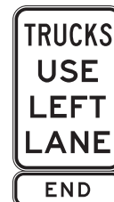
End trucks use left lane sign
