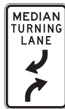
Median turning lane sign
