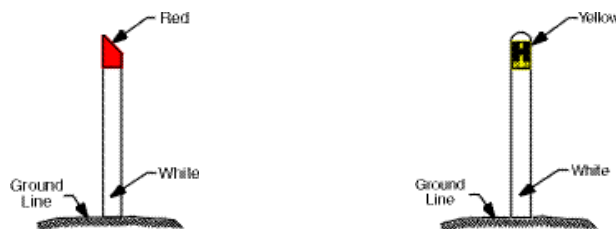
Fire hydrant indicators
