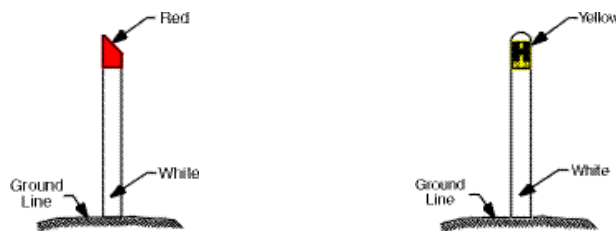
Fire hydrant indicators
