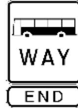
End busway sign
