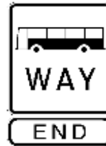
End busway sign
