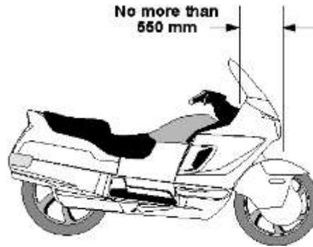
**Maximum horizontal distance from midpoint between head stem bearings of motor cycle to centre of front wheel**
