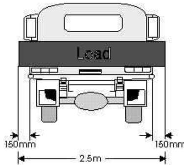
**Vehicle loaded to width limits mentioned in r. 170,
