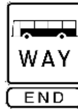
End busway sign
