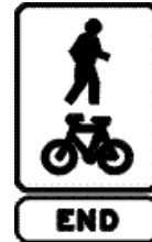
End shared path sign
