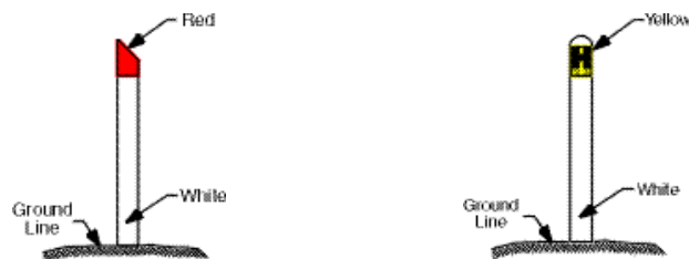
Fire hydrant indicators
