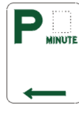
Permissive parking sign (for an area)
