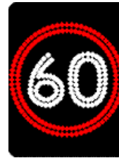
Speed limit sign (Variable illuminated sign) (circle illuminated in red)
