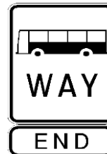
End busway sign
