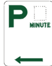
Permissive parking sign (for an area)
