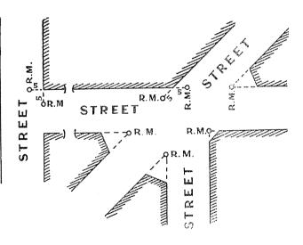
Reference Marks to be of galvanised iron tube, iron bar, or glass, and not less than half-inch diameter and 15 inches long. The upper surface of the mark shall be sunk at least six inches below the natural surface of the ground.
