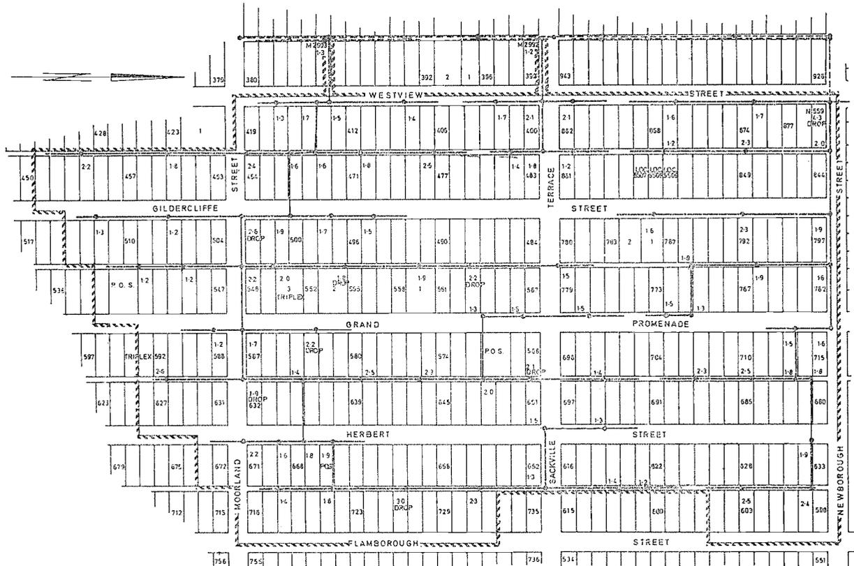
CENTRE LINE OF SEWERS AT MANHOLES TO BE ON THE 3.5m ALIGNMENT IN ROAD RESERVES & 10m ALIGNMENT IN LOTS UNLESS OTHERWISE SHOWN.
