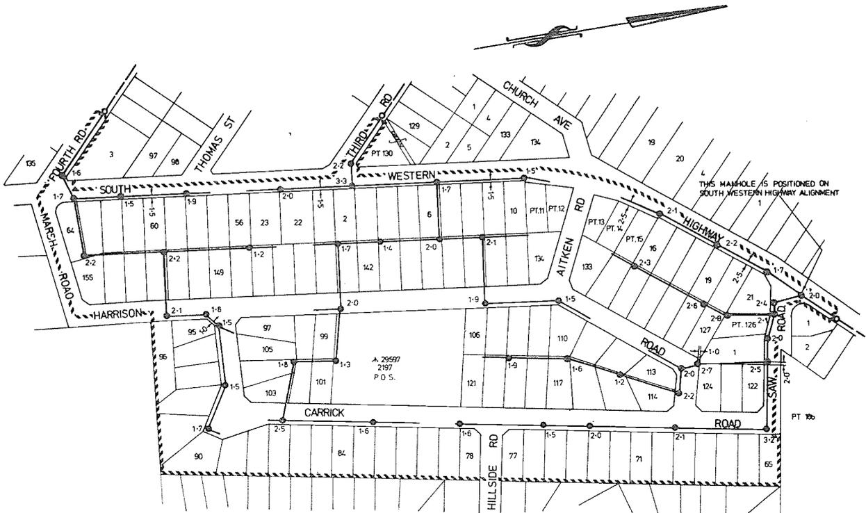
CENTRE LINE OF SEWERS AT MANHOLES TO BE ON THE 3.5m ALIGNMENT IN ROAD RESERVES & 1.0m ALIGNMENT IN LOTS UNLESS OTHERWISE SHOWN.
