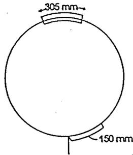
150 mm minimum distance of escape gap from Hauling rope attachment point or points. Gap not to be inserted between Hauling attachment points if there are two.
