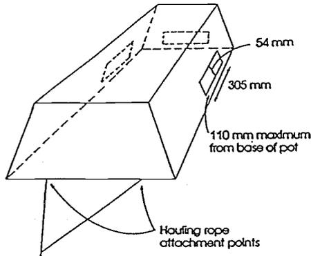
150 mm minimum distance of escape gap from hauling rope attachment point or points.
