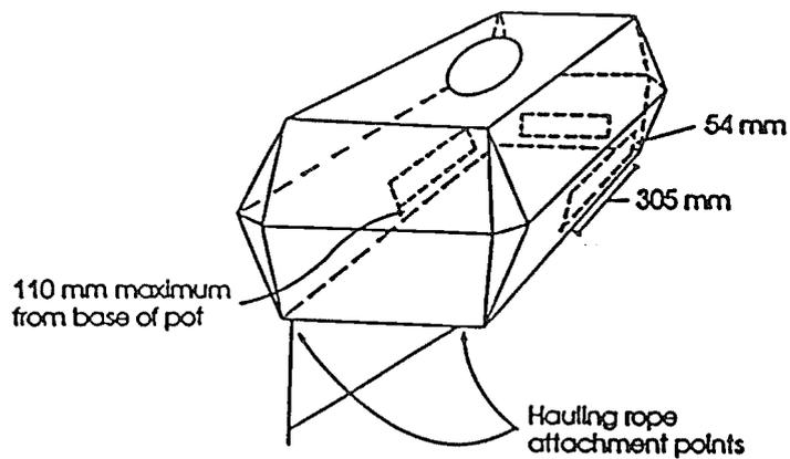
150 mm minimum distance of escape gap from hauling rope attachment point or points.
