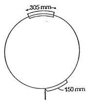
150 mm minimum distance of escape gap from Hauting rope attachment point or points. Gap not to be inserted between Hauting attachment points if there are two.
