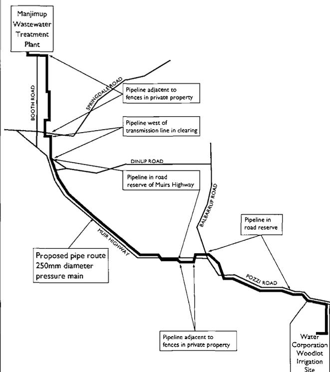
This notice of intent is for the construction of a pressure main from the Manjimup wastewater treatment plant to a woodlot on Pozzi Road. The Water Corporation is currently developing the woodlot so that treated wastewater may be irrigated and stored at the site. The project is proposed to improve the environmental impact due to wastewater disposal by re-using all the wastewater instead of disposing of it in Manjimup Creek.
