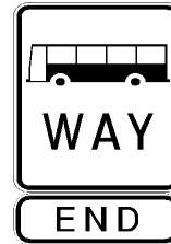
End busway sign
