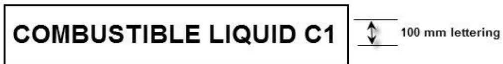
Figure 6 — Placard for C1 combustible liquids
