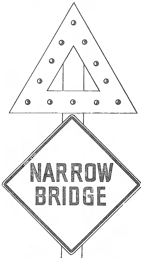
FIGURE 13.—NARROW BRIDGE SIGN.
