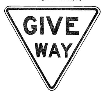
This sign shall consist of an inverted triangular metal base. side of the equilateral triangle shall be approximately 30 inches long. The sign shall have white letters and a five-eighths inch white border on a red background and the legend shall consist of the word "GIVE" in letters five inches high, and the word "WAY" in letters four inches high.
