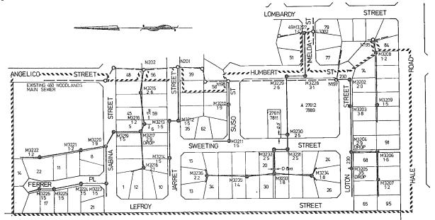
CENTRE LINE OF SEWERS AT MANHOLES TO BE ON THE 3-5m ALIGNMENT IN ROAD RESERVES & 1-0m ALIGNMENT IN LOTS UNLESS OTHERWISE SHOWN.
