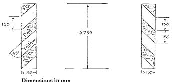
A dimension specified in the diagram for a side of the rear marking plates is a minimum dimension for that side. ".
