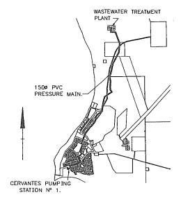
THE WATER AUTHORITY OF WESTERN AUSTRALIA PROPOSES TO CONSTRUCT A WASTEWATER TREATMENT PLANT, SEWERAGE PUMPING STATION AND A 150mm DIAMETER SEWERAGE PRESSURE MAIN.
