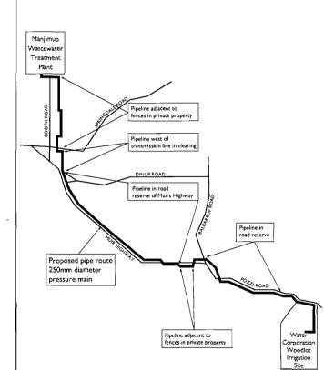
This notice of intent is for the construction of a pressure main from the Manjimup wastewater treatment plant to a woodlot on Pozzi Road. The Water Corporation is currently developing the woodlot so that treated wastewater may be irrigated and stored at the site. The project is proposed to improve the environmental impact due to wastewater disposal by re-using all the wastewater instead of disposing of it in Manjimup Creek.
