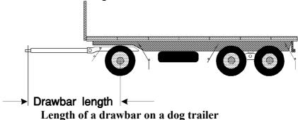
(2) The distance between the coupling pivot point on a drawbar, and the centre of the axle group or single axle on a trailer with only one axle group or single axle (except a semi-trailer) must not be over 8.5 m.
