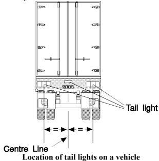
(4) Tail lights fitted in accordance with this Division may also serve as rear clearance lights if they are fitted to a vehicle in accordance with rule 87(3).
