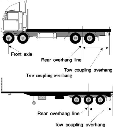
Tow coupling overhang — semi-trailer with extra coupling at rear
