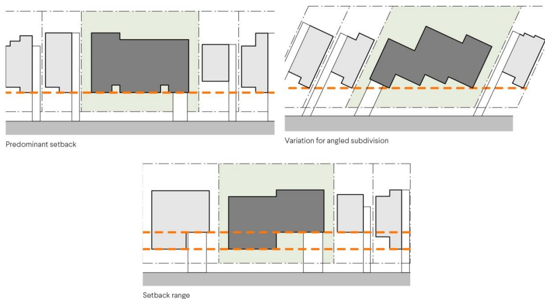
Figure 2.3a, b & c Street setbacks should be consistent with existing setback patterns in the street or setbacks that achieve the desired future character of the area.
