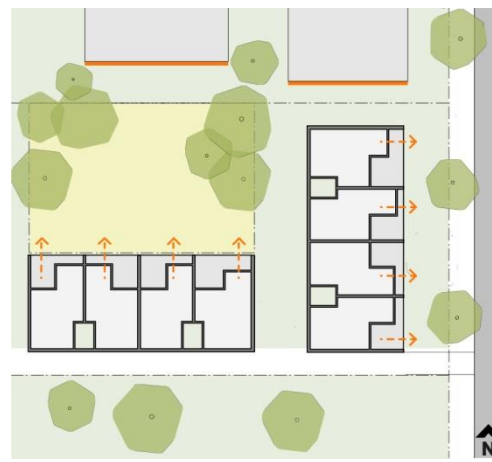
Figure 2.4b On sites with solar access to the north consider larger setbacks and locating the open space for northern orientation of units.
