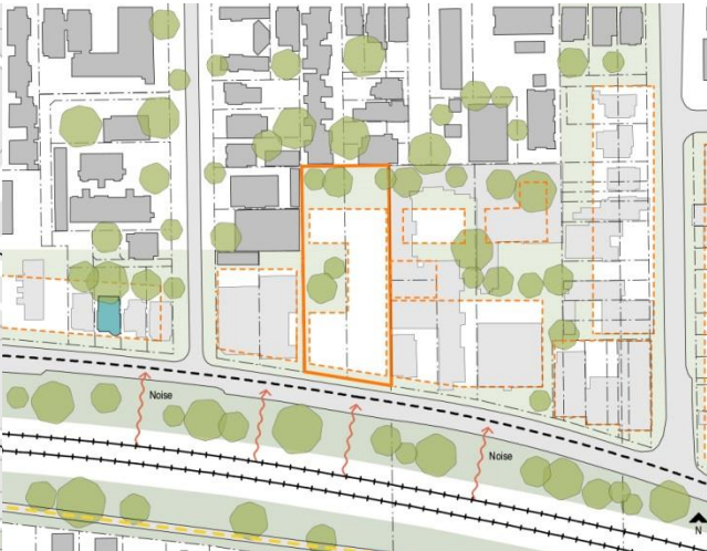
Figure A3b Site context plan Considers the character of the street(s) that the proposed development addresses, and shows its spatial enclosure by buildings or landscape elements. It should outline surrounding building uses and heights, front setbacks, pedestrian access, awnings, vehicle driveways and public domain elements including street trees, verges and footpaths. It is appropriate that all proposals for apartment buildings address this scale.
