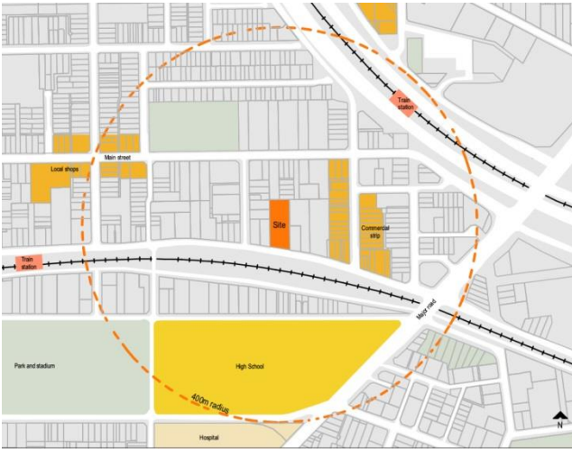
Figure A3a Local context plan Outlines the urban structure including streets and open spaces. It should also include topography contours, drainage and vegetation patterns, services and future infrastructure requirements (if known), land use zones, cadastre boundaries and identification of heritage items and other local landmarks. It is appropriate to address this scale when planning for individual or small groups of apartment building sites. A radius of 400 to 1000 metres should be considered.
