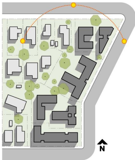
Figure 3.2a Proposed buildings are sited to clearly address the street while maximising solar access to apartments.
