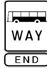
End busway sign
