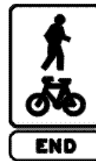
End shared path sign
