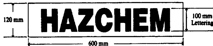
Figure 1 — Form and dimensions of an outer warning placard
