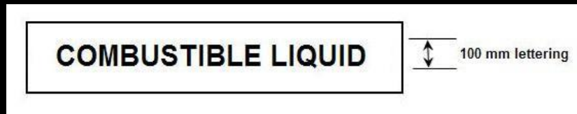
Figure 6 — Placard for C1 combustible liquids
