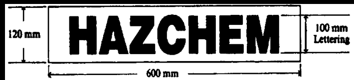
Figure 2 — Template for a placard for dangerous goods (other than C1 combustible liquids) in bulk
