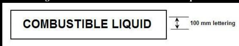
Figure 6 — Placard for C1 combustible liquids
