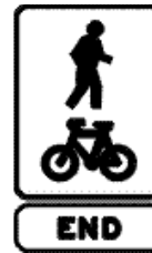
End shared path sign
