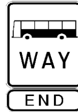
End busway sign
