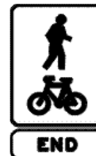
End shared path sign
