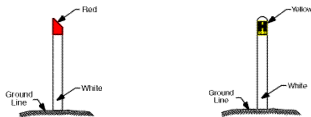
Fire hydrant indicators
