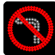
No left turn sign (Variable illuminated message sign) (circle and slash illuminated in red)
