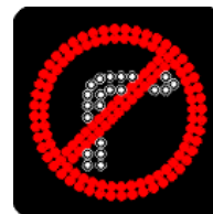
No right turn sign (Variable illuminated message sign) (circle and slash illuminated in red)
