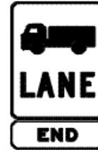
End truck lane sign
