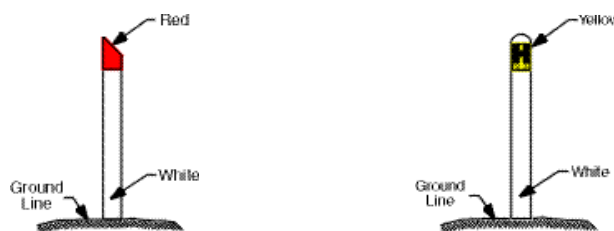
Fire hydrant indicators
