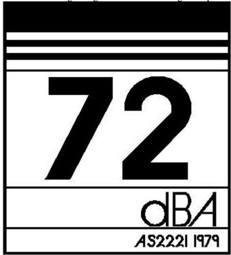
(b) Mean Sound Level — The test procedure to establish the Mean Sound Level shall be in accordance with AS 2221 Part 1 1979 —Engineering Method for Measurement of Airborne Sound Emitted by Compressor/Primemover Units Intended for Outdoor Use.
