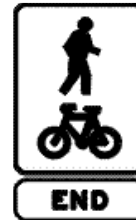
End shared path sign
