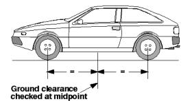
Ground clearance at the midpoint between 2 axles
