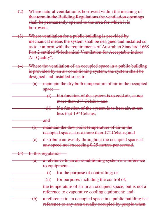
the building is in use that is between a floor, 180 cm above the floor, 60 cm from walls adjacent to the floor and 60 cm from fixed equipment that is, or forms part of, an air conditioning system.
