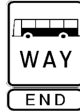
End busway sign
