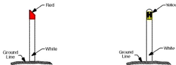
Fire hydrant indicators
