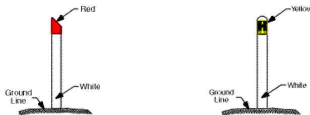
Fire hydrant indicators
