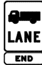
End truck lane sign
