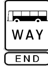
End busway sign
