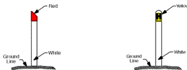
Fire hydrant indicators
