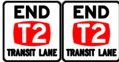
End transit lane sign (End transit lane (T2) sign) (background to "T2" in red)
