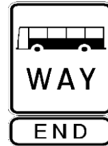
End busway sign
