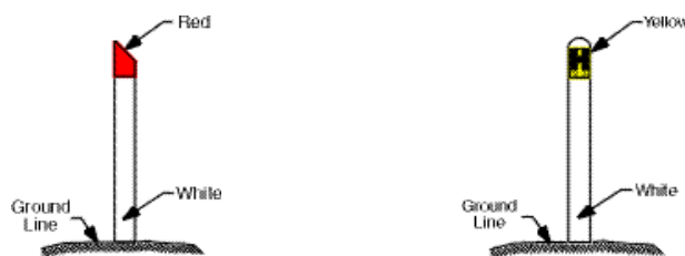
Fire hydrant indicators
