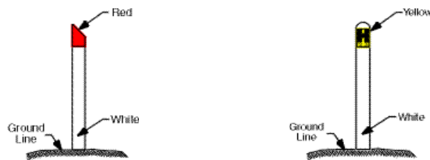
Fire hydrant indicators
