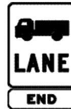
End truck lane sign
