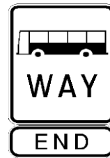
End busway sign
