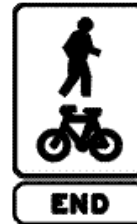
End shared path sign
